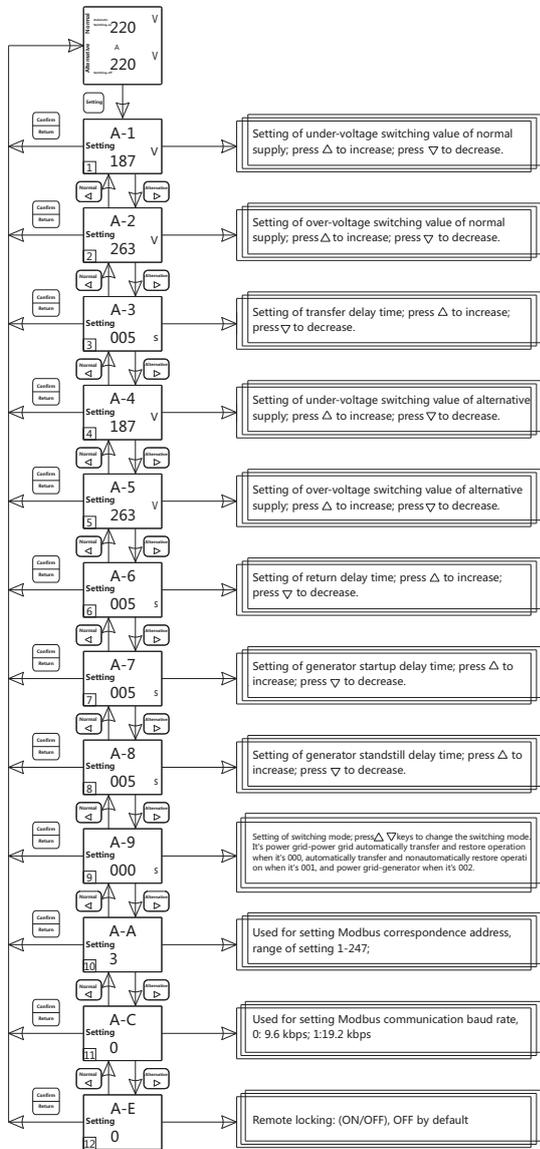
Operation interface for parameter setting of controller
