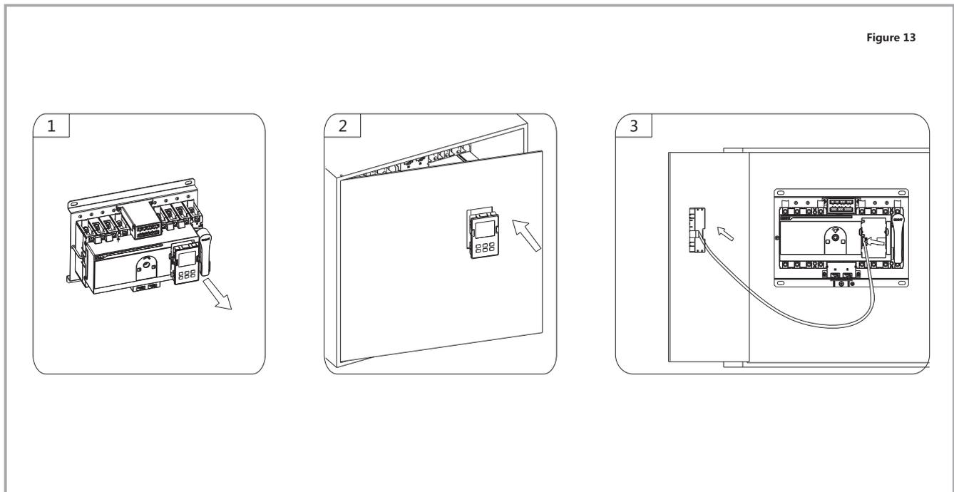
Signal and control terminal wiring
