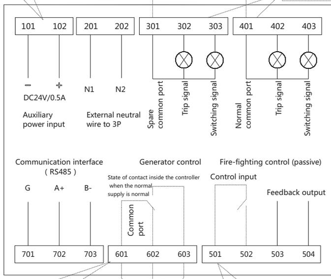
Only used in power grid-generator mode; connected with the generator based on required; when the normal supply is failure, 601 and 603 will be connected through.
